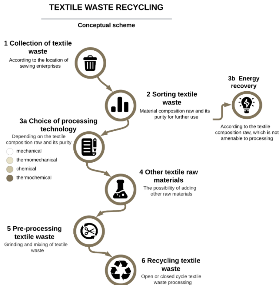
Fig. 1. Conceptual scheme of recycling textile waste
